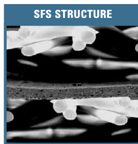
Cross-section of BLOCK-IT* 380 spunbond/film/spunbond laminate.
